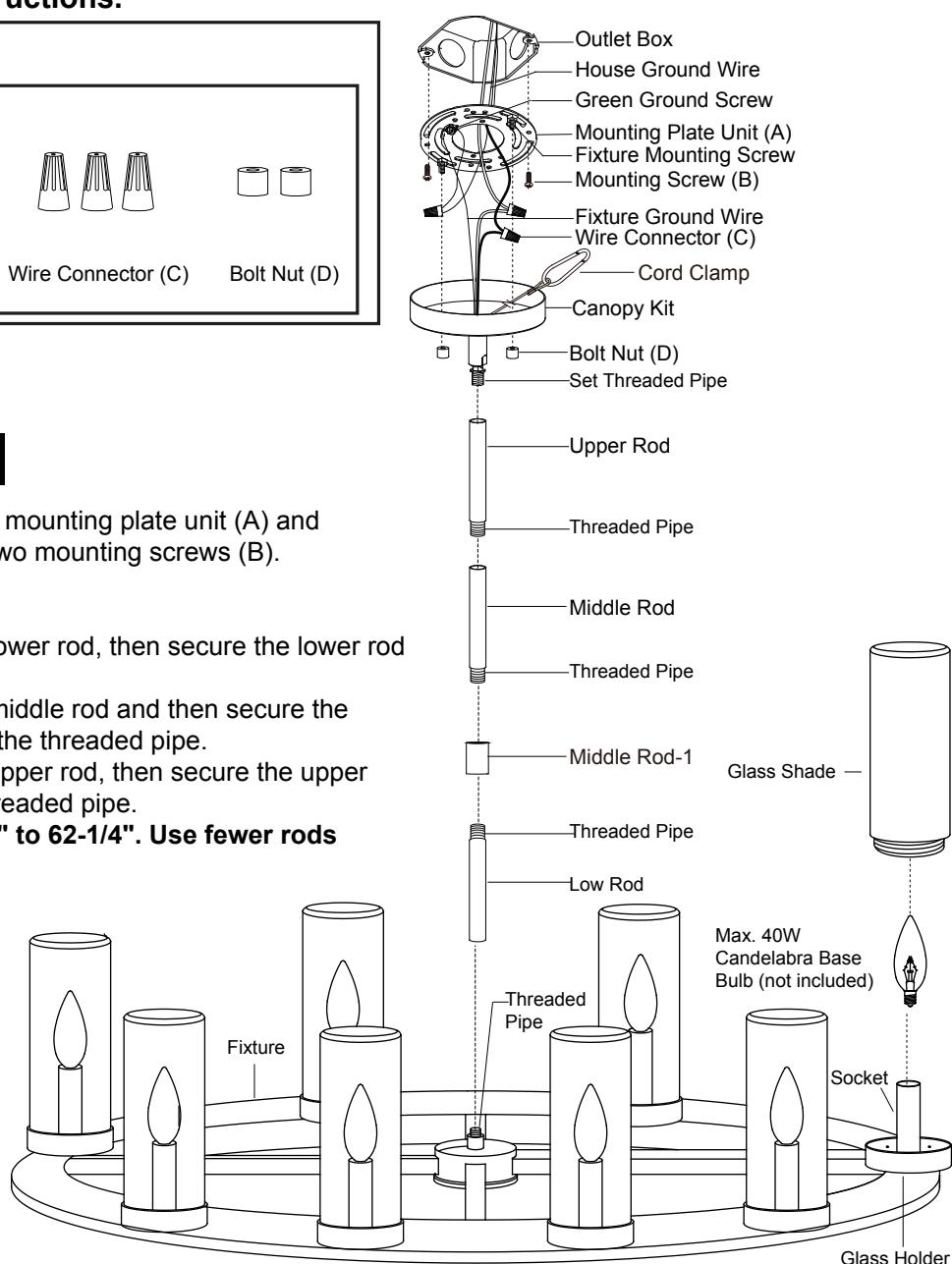
7. Install 8 x 40W Max. candelabra base bulbs (not included). See relamping label at socket area or packaging for maximum wattage allowed.
